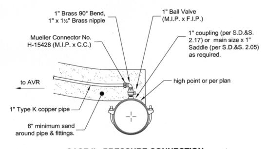
CASE II - PRESSURE CONNECTION ELEVATION
